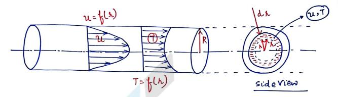
Consider a given c/s of the pipe at which the relocity distribution and the tempr distribution are as shown in the figure Consider a differential elemental ring of fluid flow in the c/s of the pipe at a radius of "i' measured from the axis. Let 'di' be the differential radius of the elemental ling then din = Differential mass flow Rate of fluid through
