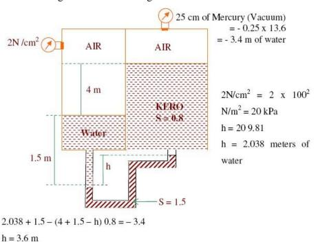
3. Compute the pressure different between 'M' and 'N' for the system shown in figure.
