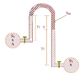
Inverted U-tube manometer is used to measure small difference in pressure between any two points. It consists of an inverted U-tube connecting the two points between which the pressure difference is required. In between there will be a lighter manometric liquid. Pressure difference between the two points can be calculated by writing the gauge equations for the system.
