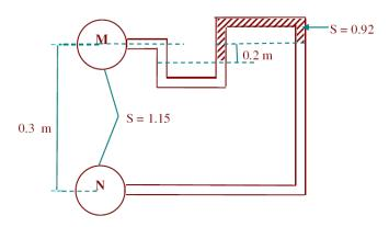
Let ' $h_M$ ' and '  $h_N$ ' be the pressure heads at M and N in m of water.
