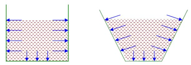
Fluid is a state of matter which exhibits the property of flow. When a certain mass of fluids is held in static equilibrium by confining it within solid boundaries, it exerts force along direction perpendicular to the boundary in contact. This force is called fluid pressure.
