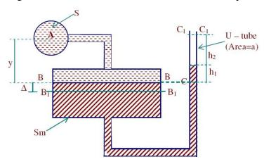
A single column manometer consists of a shallow reservoir having large cross sectional area when compared to cross sectional area of U – tube connected to it. For any change in pressure, change in the level of manometric liquid in the reservoir is small and change in level of manometric liquid in the U- tube is large.
