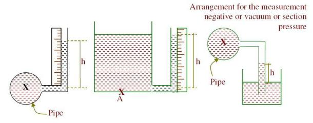
Piezometer consists of a glass tube inserted in the wall of the vessel or pipe at the level of point at which the intensity of pressure is to be measured. The other end of the piezometer is exposed to air. The height of the liquid in the piezometer gives the pressure head from which the intensity of pressure can be calculated.
