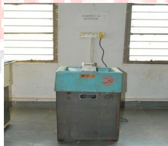
Fig 2 Jominey End Quench Test Apparatus
